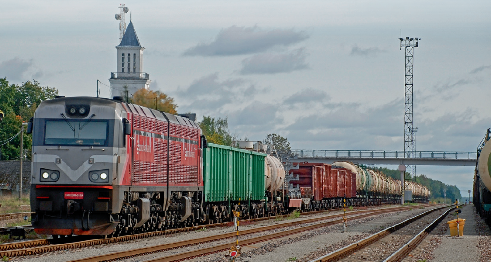
Below: LDZ Cargo 2M62UM-119 stands at Valga on the Estonia-Latvia border with a long freight bound for Latvia on 18 September 2020. These locos were rebuilt from Soviet era 2M62 locos by CZ Loko from 2015 onwards and are equipped with MTU engines, providing a total output of 4.4 MW.
