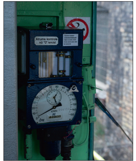
Above: Soviet era train event recorder on a diesel shunter at Ventspils depot.
