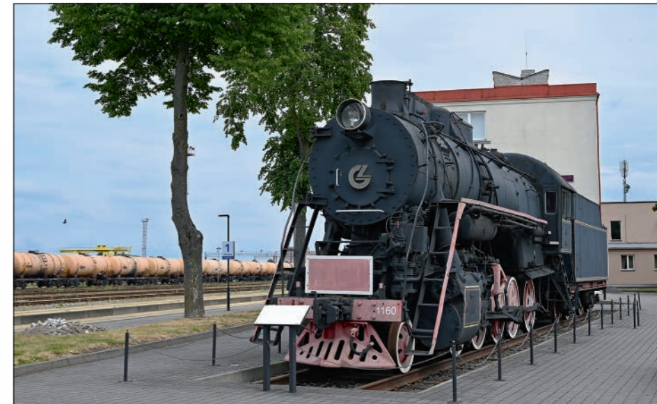
Above: 2-10-0 steam loco L-1160 (BMZ Bryansk 1160, 1949) is plinthed outside the station at Klaipėda.
